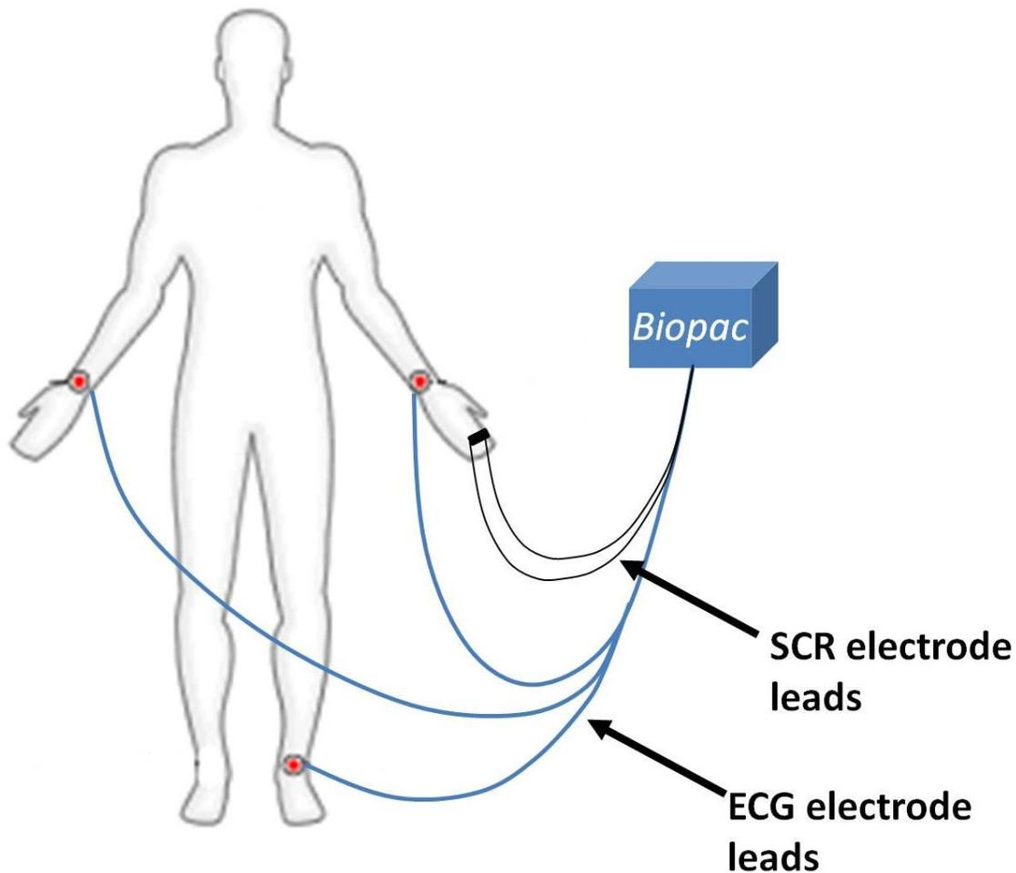
**Figure 5.1** Physiological acquisition setup for skin conductance response collection
